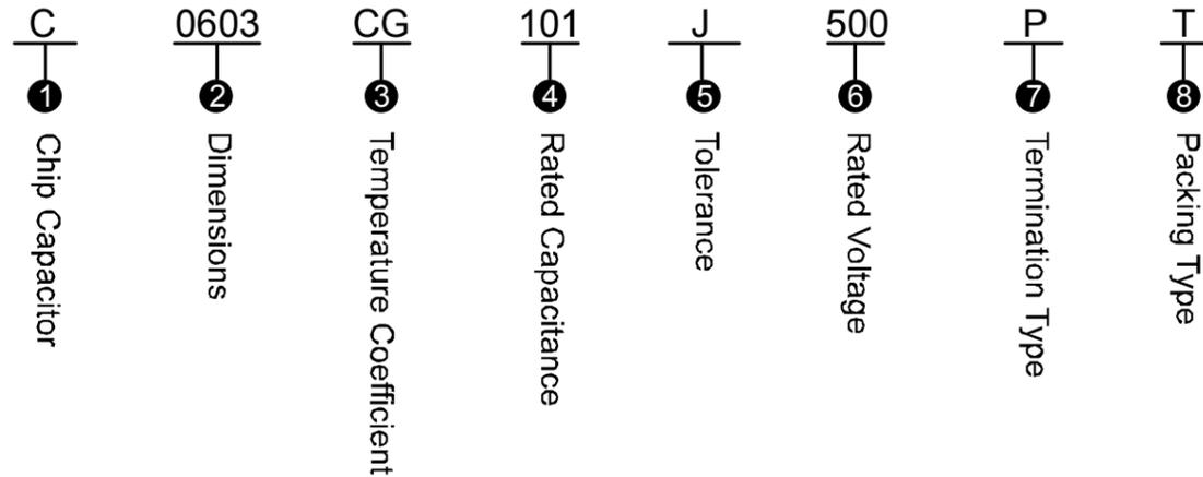
① C: General Purpose Non-Magnetic Multilayer Ceramic Capacitors
