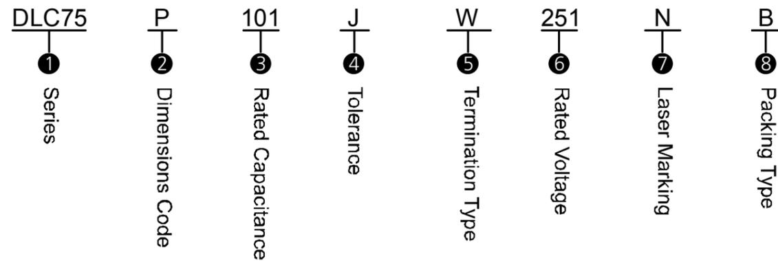
① **Series:** Dalicap 75 Series Low ESR Microwave Capacitor, Temperature Coefficient:  $0 \pm 30$ ppm/°C.
