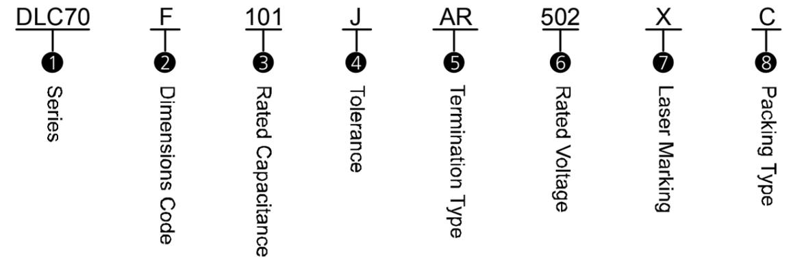
① **Series:** Dalicap 70 Series High RF Power Capacitor, Temperature Coefficient:  $0 \pm 30\text{ppm}/^\circ\text{C}$ .
