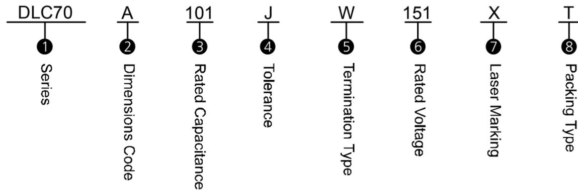
① **Series:** Dalicap 70 Series High Q High Power Capacitor, Temperature Coefficient:  $0 \pm 30\text{ppm}/^\circ\text{C}$ .
