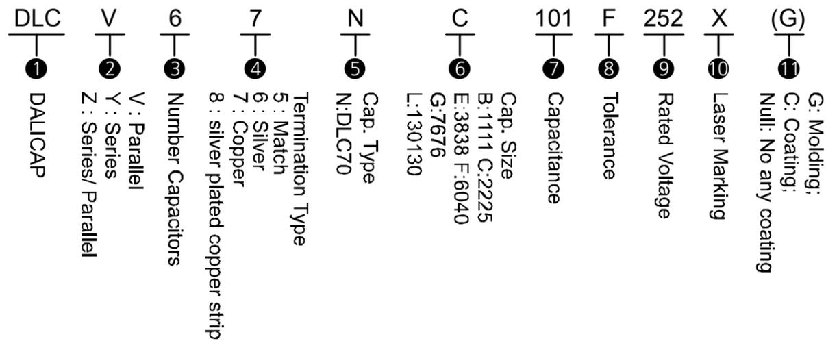
Capacitance: For capacitor values requiring 3 significant digits,
